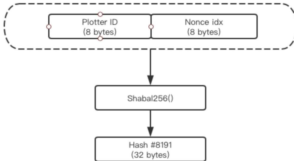
Based on computing the Plotter ID and Nonce idx through Shabal256(), hash #8191 will be generated. Hash #8191, Plotter ID and Nonce idx will then be used in the next round of Shabal256() encryption to become a new hash, Hash #8190 (as shown below).
