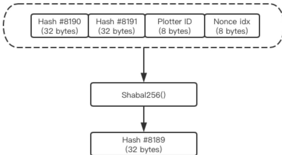
From the calculation of hash #8064, the length of input strings being added will exceed 4096 bytes. New input strings will thus be added in the form of Shabal256() hashed entries. This process will be performed until hash #0 is calculated (as shown below).
